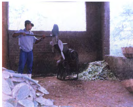
b. Small electrical chopper (Brazil)
