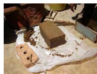
Step 5. UMB ready for drying
